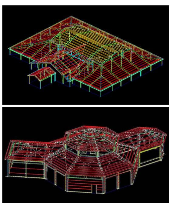
**Figure 4** .Two more examples of building designs automatically generated by RCC's Design++ based systems. (Courtesy: Robertson Ceco Corporation)
