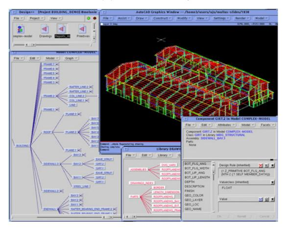
Figure 2. A screenshot of the Design++ interface, showing parts of RCC's knowledge capture of metal building design, the core super model, and the 3D model of a specific building that was automatically generated by the system. (Courtesy: Design Power Inc.)
